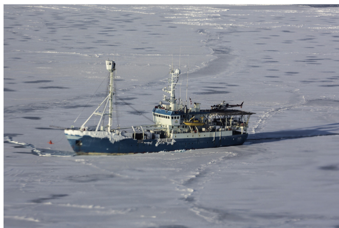
Fig. 1. RV Lance during the field experiment in the Barents Sea, 24 March 2014. The EM system at the bow is visible by its red color. Photograph taken from Polar 5 aircraft by Stefan Hendricks. (For interpretation of the references to color in this figure legend, the reader is referred to the web version of this article.)
